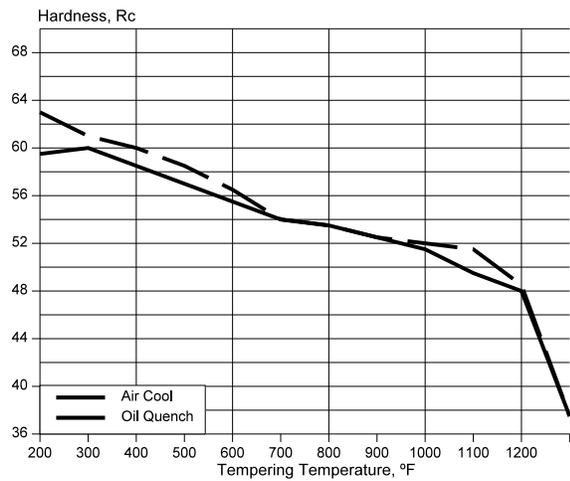
Test samples 1" round x 2" long were hardened by air and oil quenching from 1725°F and tempered at the indicated temperatures. Resulting hardness is shown above.
